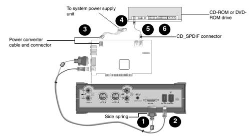
Figure 2-5: Connecting the cables to the audio card.
